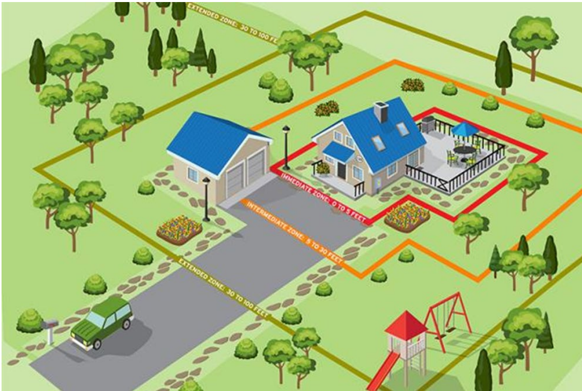
Image 2. Defensible space around the home. Courtesy of the National Fire Protection Association – provided by U.S. Forest Service.
